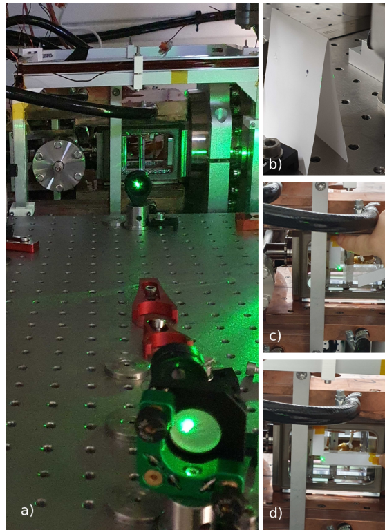
Figure 4.18: The alignment of the SC. In a) the laser which represented the probe-control-setup is shown. With this laser, the SC is aligned. The back reflections on the edge of a paper are shown in b). The position alignment is shown in c) and d) for the z-axis position and the y-axis position, respectively.
